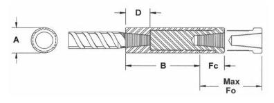
A = Diameter B = Length of Coupler Body D = Bar Engagement Fc = Connector Closed Position Max. Fo = Connector Fully Open Position
