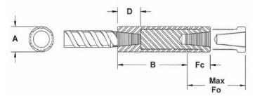
A = Diameter B = Length of Coupler Body D = Bar Engagement Fc = Connector Closed Position Max. Fo = Connector Fully Open Position
