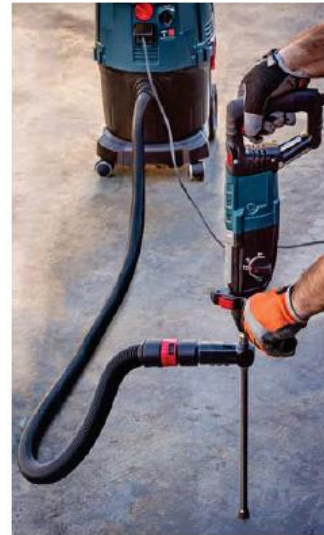
Bosch/Simpson Strong-Tie DXS drill bit used with the vacuum dust extraction system described in Section 3.2.3.2
