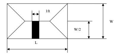
3. The calculation to determine sealant surface contact required, referred to as "bite" is as follow:
